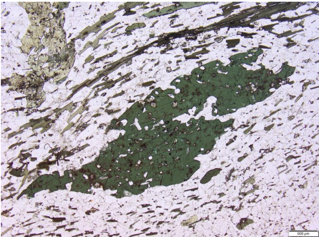
Figure 33. 225476a_dextral Hbl fish wrapped by Bi-ttn fabric, Ep inclusions in Hbl and in matrix - PPL
